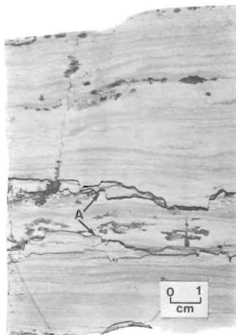
FIGURE 12: Laminated Lime Mudstone Facies Roxy et al Waskada 9-26-1-26 WPM; core slab (note: stylolites (A) ).
