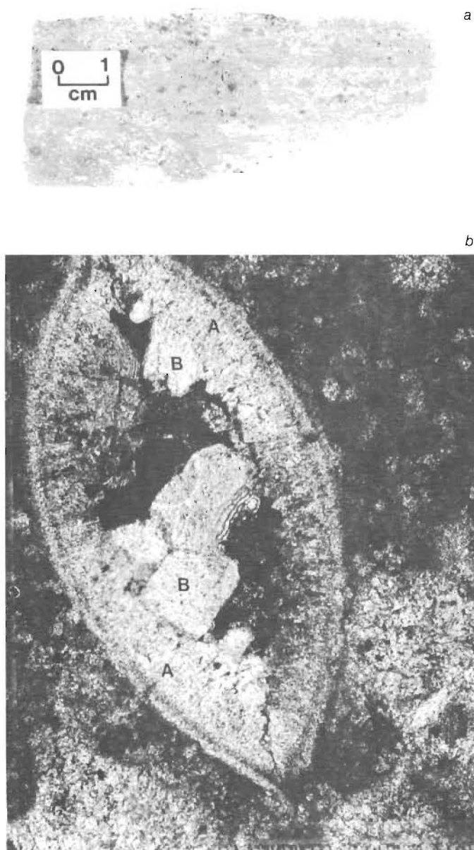
FIGURE 11: Bioclastic-Intraclastic Wackestone-Packstone Facies (a) Chevron Waskada 16-13-1-26 WPM; core slab (b) Ostracod: primary void space partly in-filled with two generations of calcite cement: (A) drusy; (B) blocky (Newscope S. Waskada 13-7-1-25 WPM; Depth 939.8 m; Thin Section X 2.5)
