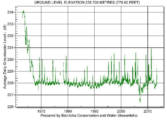
Figure 5 - Provincial Red River Floodway monitoring station near the floodway embankment. The construction of the floodway lowered the water table in its vicinity toward a groundwater base level determined by the base of the channel. The water table dropped six metres during initial construction and then stabilized. Expansion of the Floodway from 2005 to 2009 matches a drop of about 1.5 m in the hydrograph, likely caused by dewatering during the construction phase.
