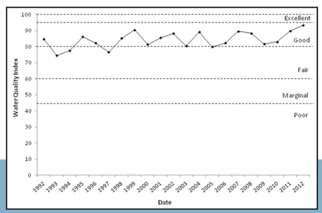
Figure 9: Water Quality Index calculated from 1992 to 2012 for the Rat River at PR 303 at Otterburne
