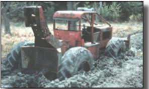
Rutting and soil compaction
