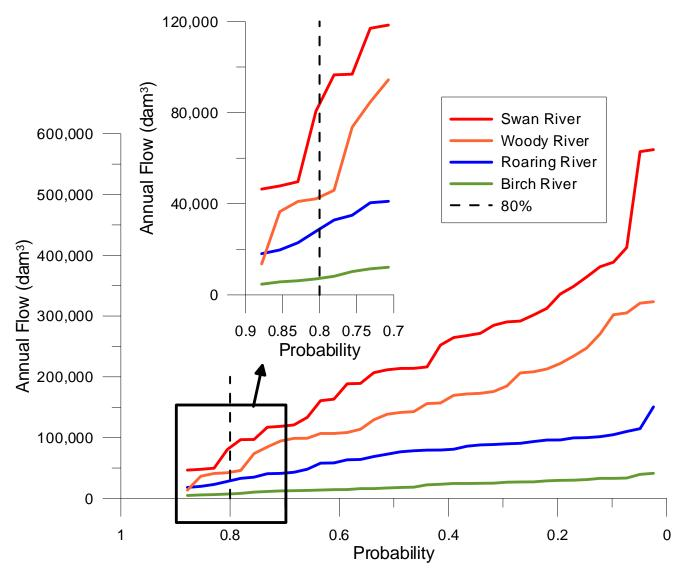
Figure 15: Flow duration curves at the gauges on Swan, Roaring, Woody and Birch rivers for the time series 1973 – 2009. Water production is taken to be the flows that are not exceeded 80% of the time.
