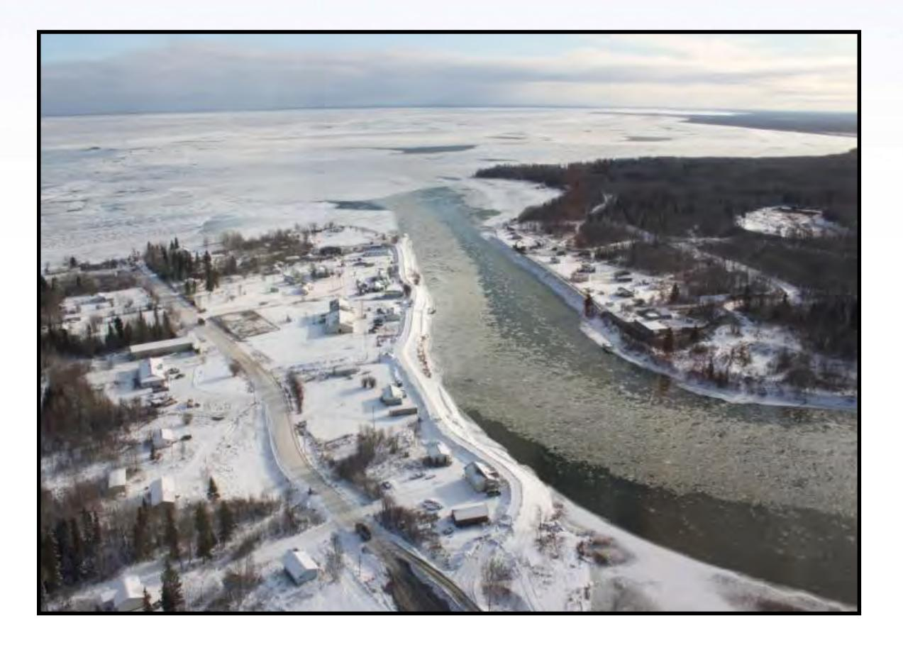
If the emergency channel had not been constructed flows through the Fairford Control Structure would have been reduced over the winter period. Lake level simulation indicate that levels on Lake Manitoba in the summer of 2012 would have been 0.4 metres higher than recorded, and summer levels on Lake St. Martin would have been 0.5 metres higher.
