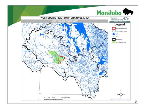
The drainage area of the creeks and rivers of the WSR IWMP extend into Saskatchewan. The creeks travel in a southeast direction through the WSR IWMP before discharging to various points into the Souris River. The total drainage area (shown in green) of the tributaries draining through the WSR IWMP is 13,330 km<sup>2</sup>, while the IWMP area alone is 4320 km<sup>2</sup>.
