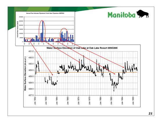
The figure shows the levels on Oak Lake from 1954 to 2000. During this period the lake was highest in April 1976 (430.76 m.a.s.l.) and lowest in February 1990 (427.84 m.a.s.l.). Each year the lake level fluctuates as levels increase in during the spring melt and then decrease as water leaves via Plum Creek and evaporation.
