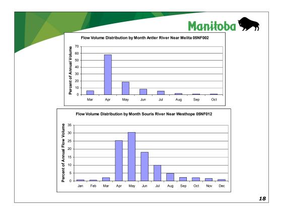
Monthly distribution of flow are shown in the figures. The pattern of flow in the Antler River is typical of the other streams in the WSR watershed. Flow is concentrated into the spring melt and no flow, or very little flow, is experienced in the winter months.
