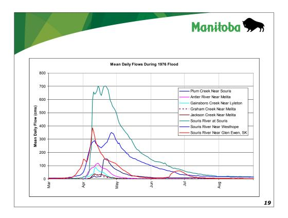
At all stations the largest annual flow volumes and the highest peak flows were observed in 1976. Flow data for 1976 was extracted from many of the stations and plotted on the figure shown.
